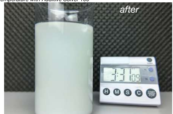
Dissolving support material at room temperature with Additive Solver 100
