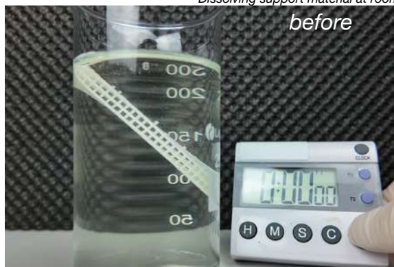
Dissolving support material at room temperature with Additive Solver 100
