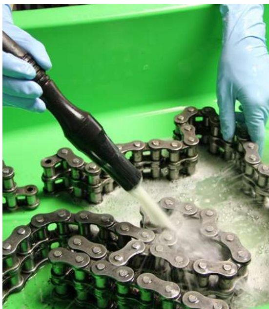
Cleaning of oil-contaminated parts in the BIO-CIRCLE GT-i
