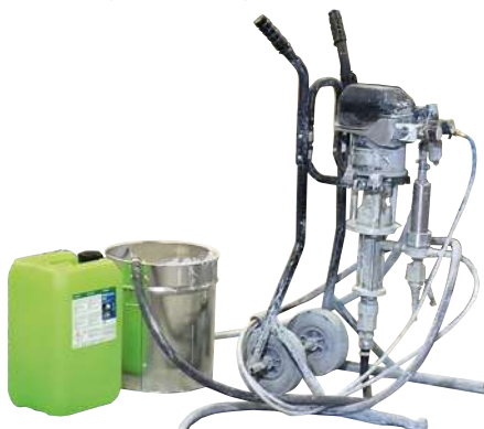
Hose system cleaning with PROLAQ Liquid
