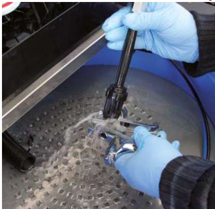
Manual or automatic cleaning of a spray gun in the PROLAQ Auto
