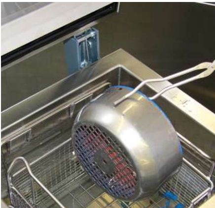
Cleaning components with PROLAQ L US in an ultrasonic cleaner
