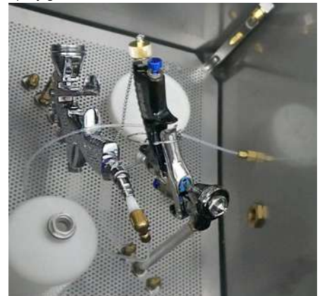
Manual or automatic cleaning of a spray gun in the PROLAQ Auto
